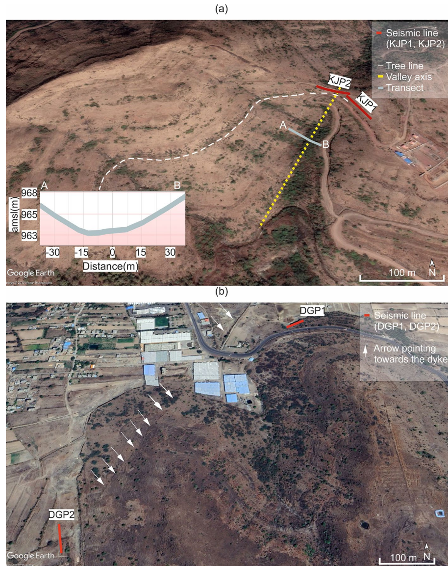
Fig. 14. 3D perspective view of Katraj and Dive Ghat study areas, where red lines represent the 2D seismic survey profiles. (a) Katraj study site where the dashed white line represents a tree line that follows the redbole layer; the yellow line represents the dyke passing along the valley, causing an asymmetrical development of vegetation around the axis of the valley; the elevation of the AB transect across the valley shows a symmetrical profile of the valley. (b) Dive ghat study site, where the white arrows point towards the signature of dyke observed in the image.
