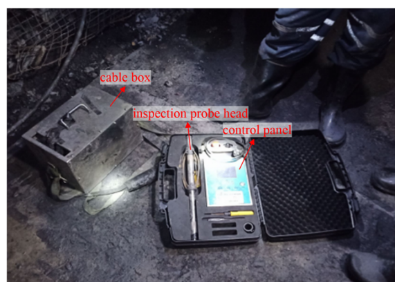
(b) Borehole visual inspection method
