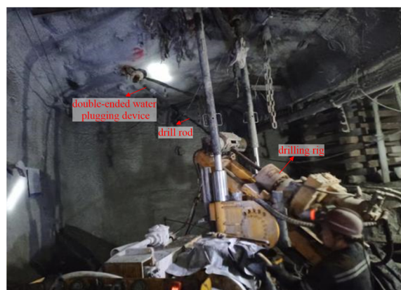
(a) Double-end water blocking leakage testing method
