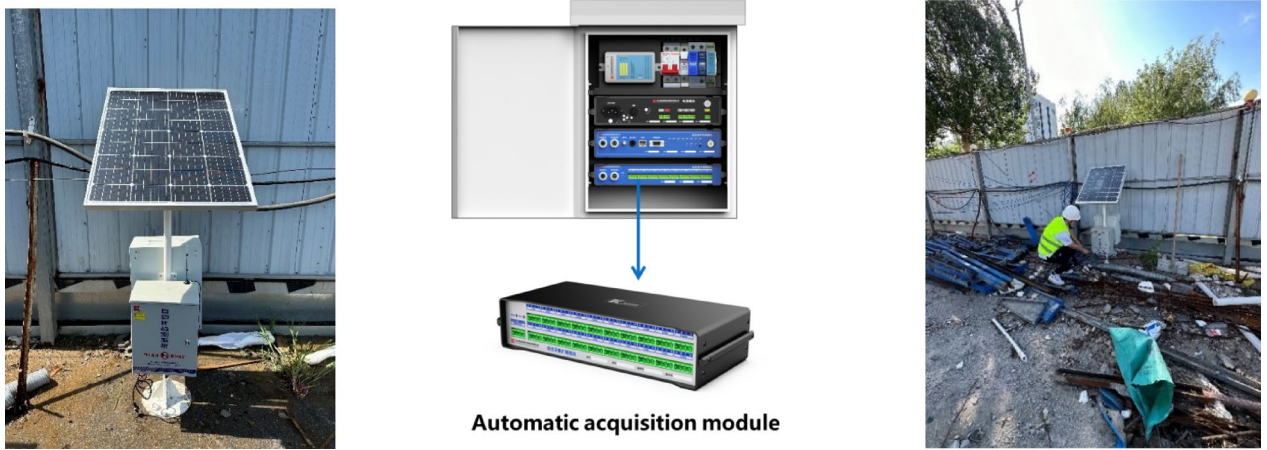
Fig. 17. Connection automatic detection system.
