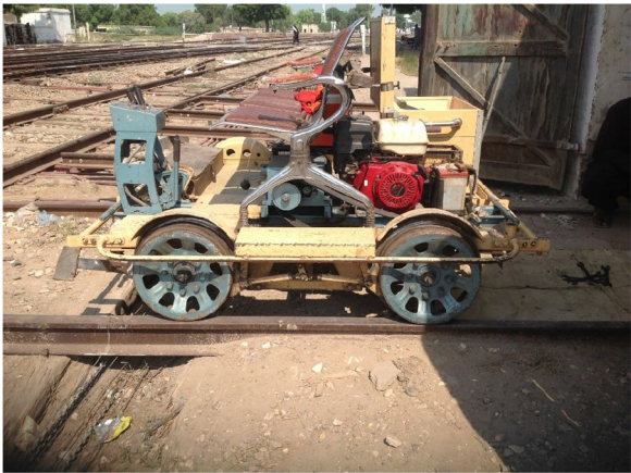
Fig. 1. Mechanical railway cart used for data collection.
