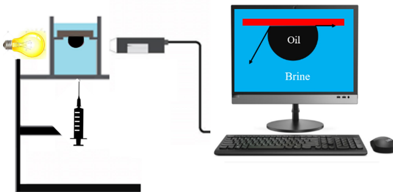
Fig. 5. Schematic representation of contact angle measurement set up using sessile drop method.
