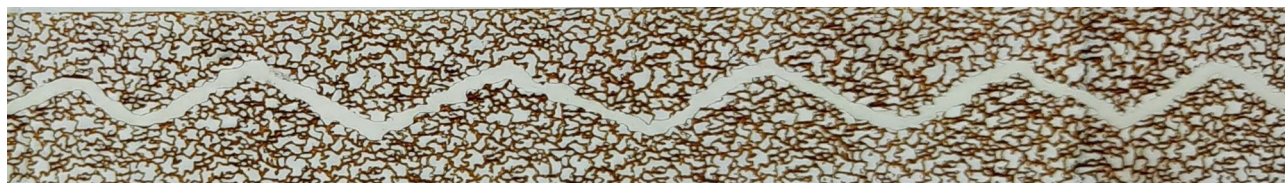
Fig. 18. Distribution of phases at the end of secondary injection of 2xcSW + 1000ppm HPAM.
