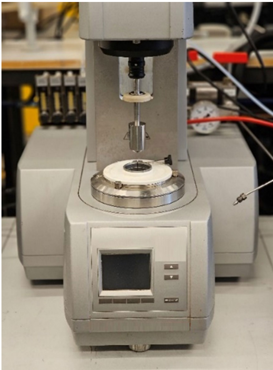
Fig. 3. Rheometer used to measure the rheological characteristics of the brine solutions.
