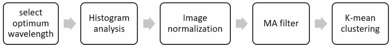
Fig. 4. Image analysis and processing steps for enhancing the detection of drone composite materials.
