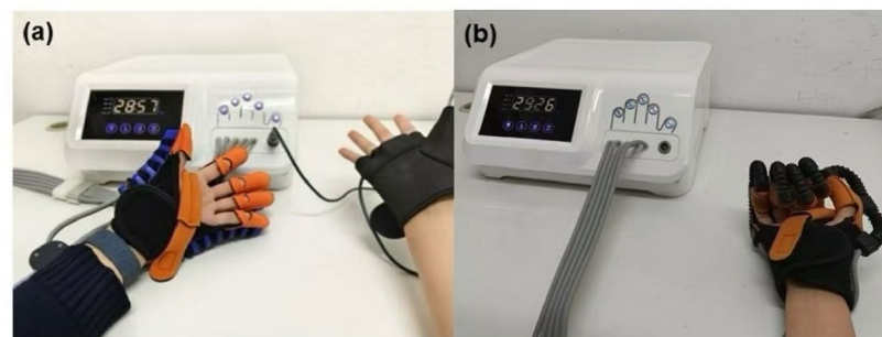
Fig. 1. Rehabilitation robot. (SRT Pavlov H1000, Beijing Softbody Robotics Technology Co., Ltd., China). (a) Mirror therapy mode; (b) Passive training mode.
