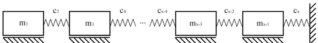
Fig. 1. A cascade system with an infinite number of degrees of freedom, consisting of inertial and elastic elements, with one side constrained.
