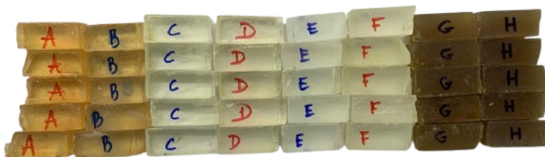
Fig. 9. Illustrates three-point bending specimens with 100% of the resins, listed in Table 6, after the flexural test.
