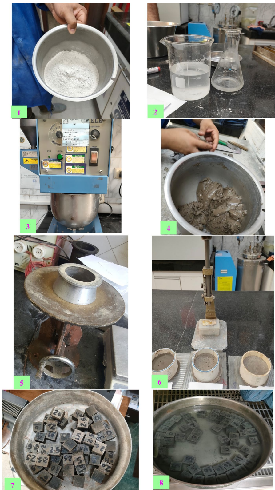
Fig. 5. A visual representation of the experimental work. Note: 1,2, weighting precursors, activator, and extra water; 3,4, mixing; 5, measuring flowability; 6, measuring setting time; 7,8, curing in air and water; 9, measuring compressive strength; 10, measuring drying shrinkage.
