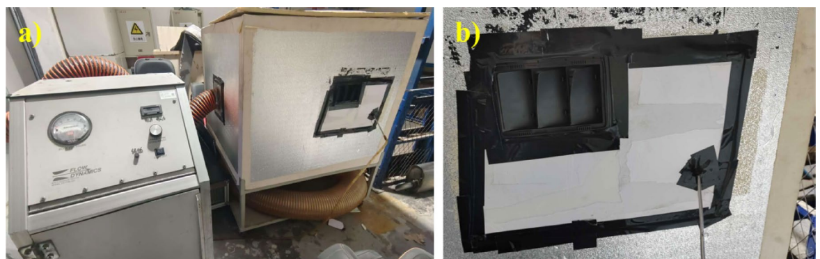
Fig. 7. (a) pressure relief valve test and (b) partial enlarged view of the pressure relief valve.
