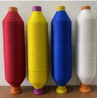
Fig. 5. Schematic of the four primary-colored rovings with a standardized linear density of 450 tex (0.45 g/m) and a twist of 680 tpm.
