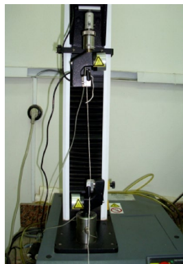
Fig. 4. Knot-pull Strength Test.
