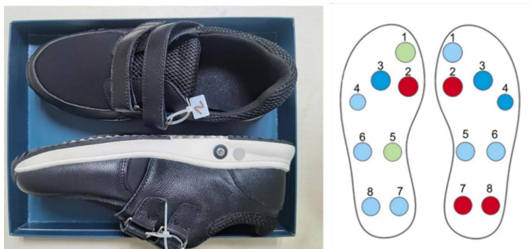
Fig. 1. Appearance of the wearable footwear system and sensor locations.
