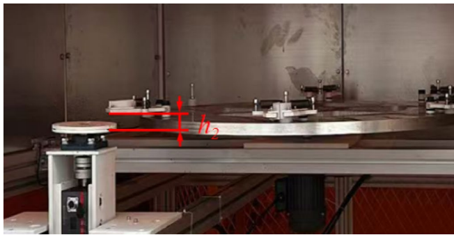
Fig. 16. Schematic diagram of enoki mushroom cutting height.
