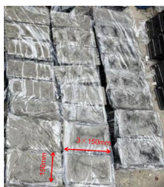
Fig. 6. Preparation and maintenance of test specimens.
