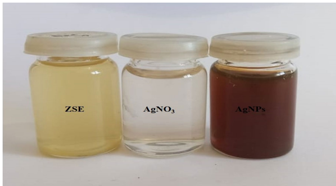
Fig. 2. Visual analysis of the change in color of the \text{AgNO}_3 solution to brown that confirms the green-synthesis of AgNPs. Key: ZSE: Z. pentandra stem extract.
