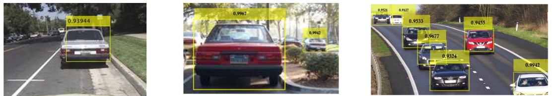
Fig. 16. Confidence scores for vehicle detection using ResNet-50 based Faster R-CNN using sgdm solver, Th = 0.3 and learning rate = 10^{-5} .
