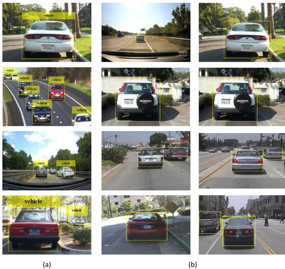
Fig. 9. Sample images from the dataset with (a, b) anchor boxes and (b) labels for vehicle detection using Faster R-CNN.
