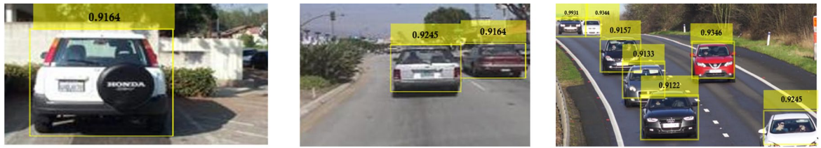
Fig. 28. Confidence scores for vehicle detection using ResNet-50 based Faster R-CNN using adam solver, Th=0.3 and learning rate = 10^{-5} .
