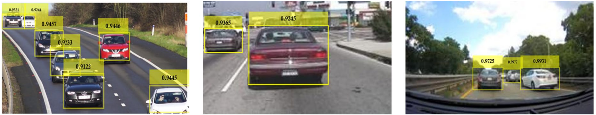
Fig. 22. Confidence scores for vehicle detection using ResNet-50 based Faster R-CNN using rmsprop solver, Th=0.3 and learning rate = 10^{-5} .
