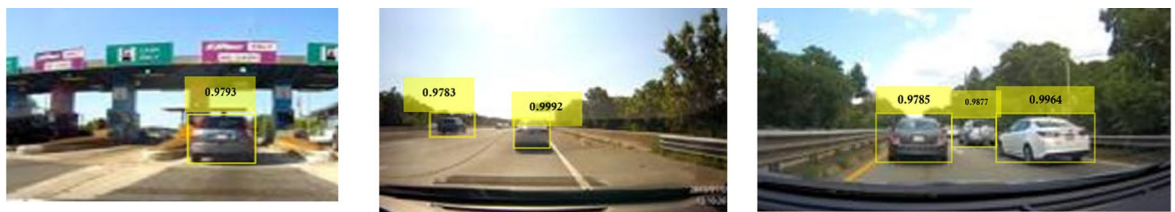
Fig. 30. Confidence scores for vehicle detection using ResNet-50 based Faster R-CNN using adam solver, Th=0.2 and learning rate = 10^{-5} .
