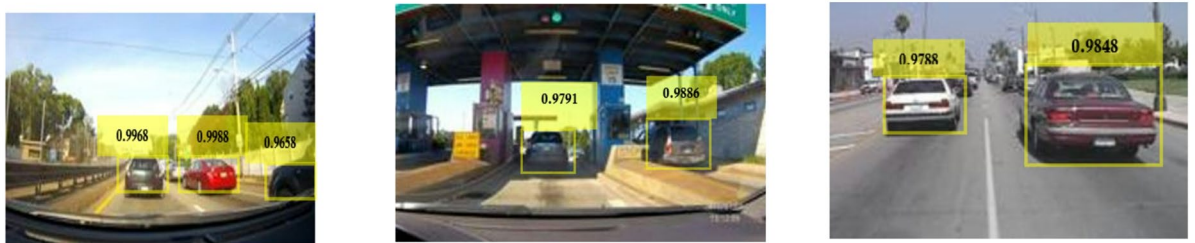
Fig. 32. Confidence scores for vehicle detection using ResNet-50 based Faster R-CNN using adam solver, Th=0.1 and learning rate = 10^{-5} .
