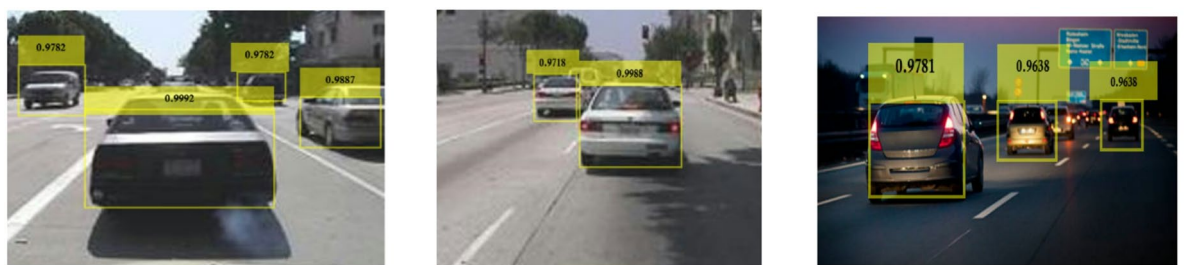
Fig. 20. Confidence scores for vehicle detection using ResNet-50 based Faster R-CNN using sgd solver, Th=0.1 and learning rate = 10^{-5} .
