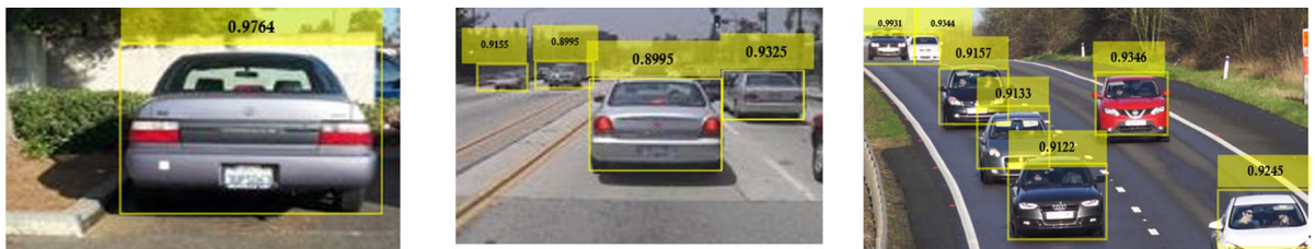
Fig. 18. Confidence scores for vehicle detection using ResNet-50 based Faster R-CNN using sgdm solver, Th = 0.2 and learning rate = 10^{-5} .
