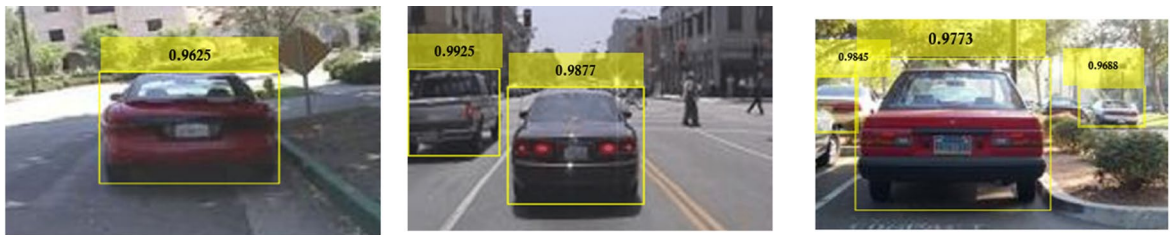
Fig. 24. Confidence scores for vehicle detection using ResNet-50 based Faster R-CNN using rmsprop solver, Th=0.2 and learning rate = 10^{-5} .
