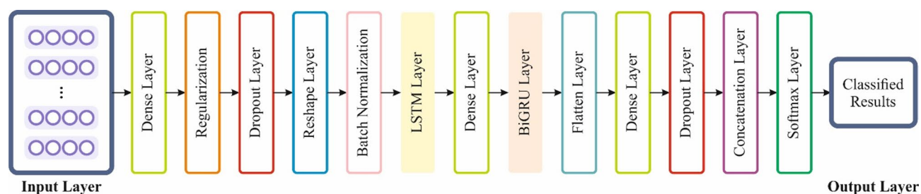
Fig. 3. Structure of the LSTM-BiGRU technique.
