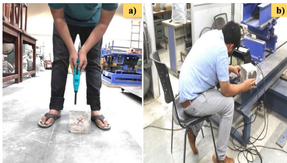
Fig. 9. Non-destructive test (a) RH, (b) UPV.
