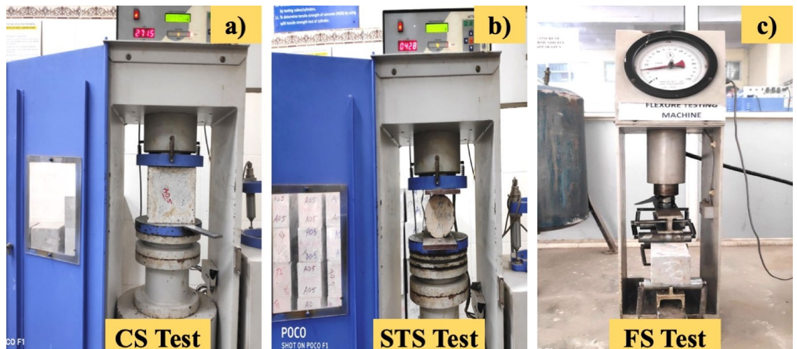
Fig. 8. Testing of casted specimens (a) CS Test, (b) STS Test, and (c) FS Test.
