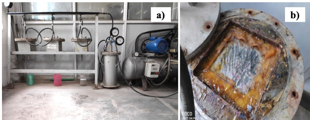
Fig. 16. (a) Water permeability test apparatus and (b) concrete cube specimen placed in water permeability test apparatus.
