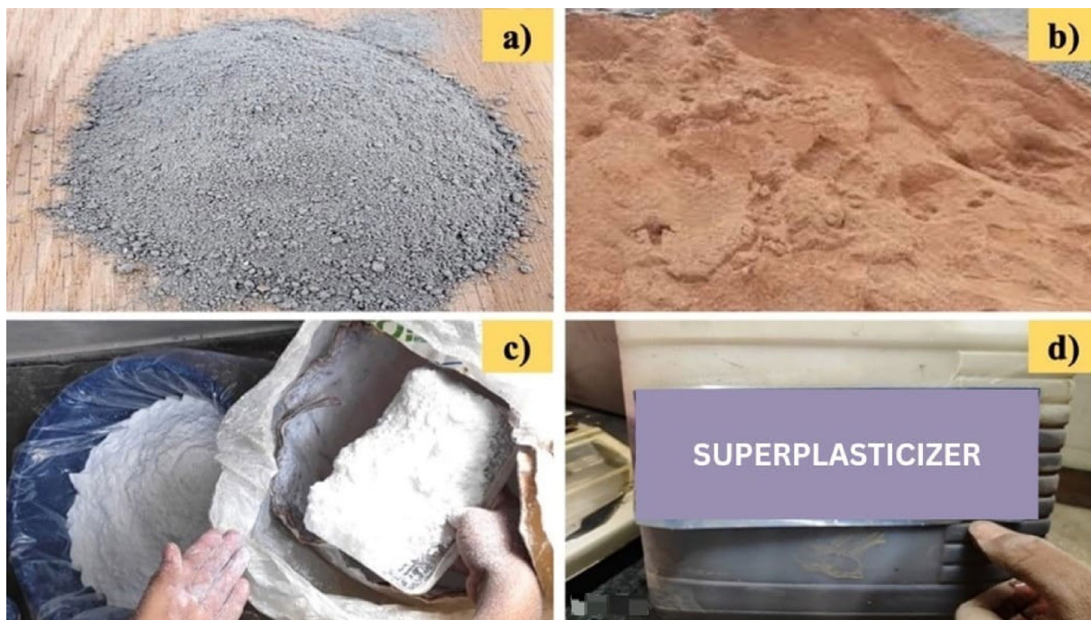
Fig. 2. Material used (a) cement, (b) Badarpur sand, (c) NT, and (d) superplasticizer.
