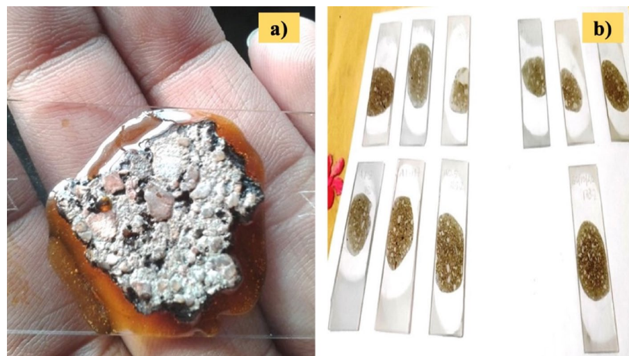
Fig. 6. The slides prepared for different dosages of NT for microscopic investigation.
