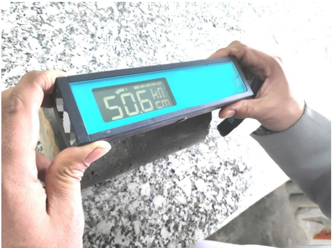
Fig. 12. SR test using a four-point Wenner probe.
