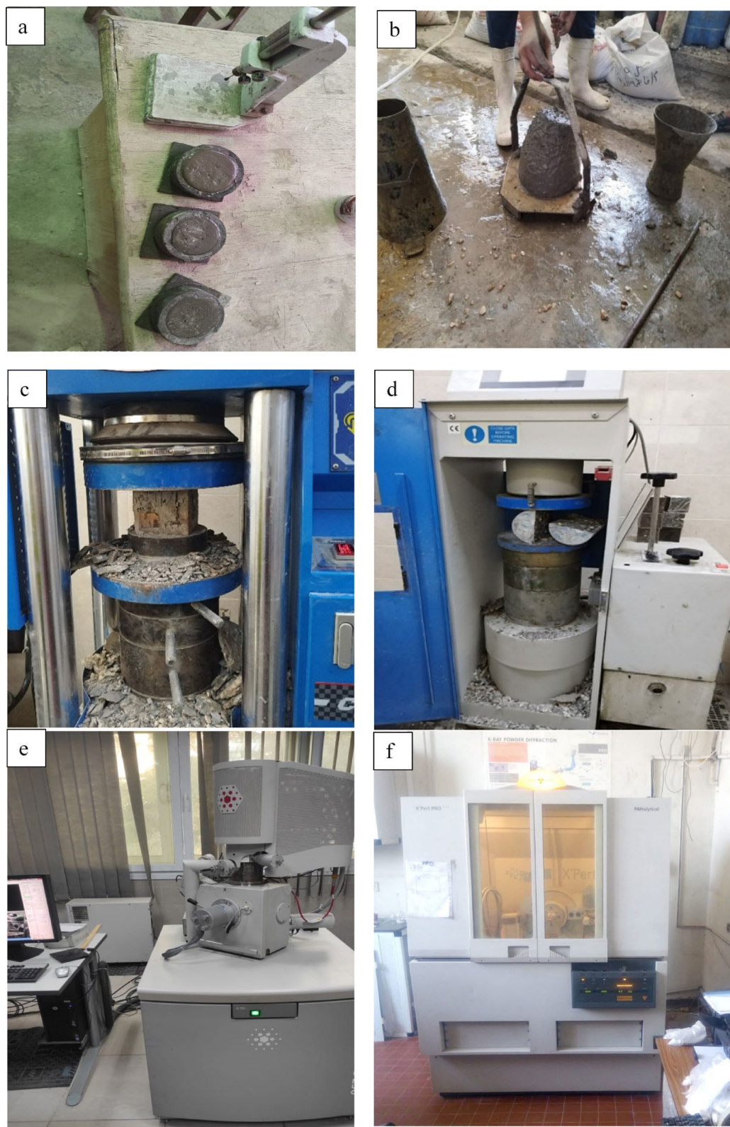
Fig. 6. Testing producer for (a) Vicat needle, (b) Slump cone test, (c) Compressive strength machine, (d) Tensile strength machine, (e) SEM &EDX analysis apparatus, and (f) XRD analysis apparatus.
