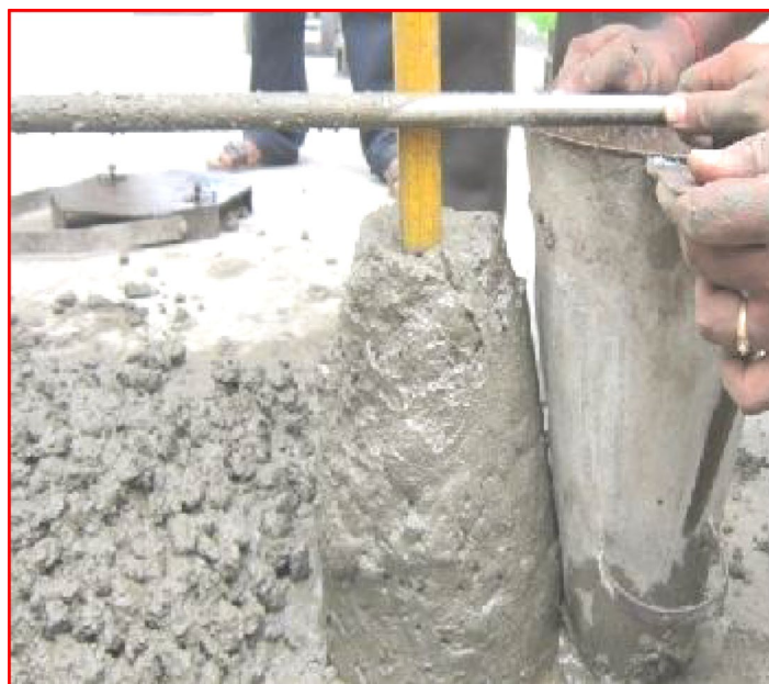
Fig. 6. Slump Test on Concrete.
