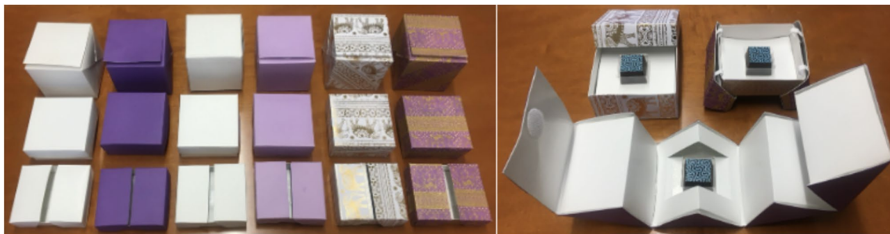
Fig. 9. The 18 boxes used in this experiment: (Left picture) Top to Down: Snail-Fold, Lift-Off, and Slide-and-Tilt; left to right (White and Purple): Smooth, Raised Dots, and Embossed Pattern. (Right picture) The three boxes in the opened position.
