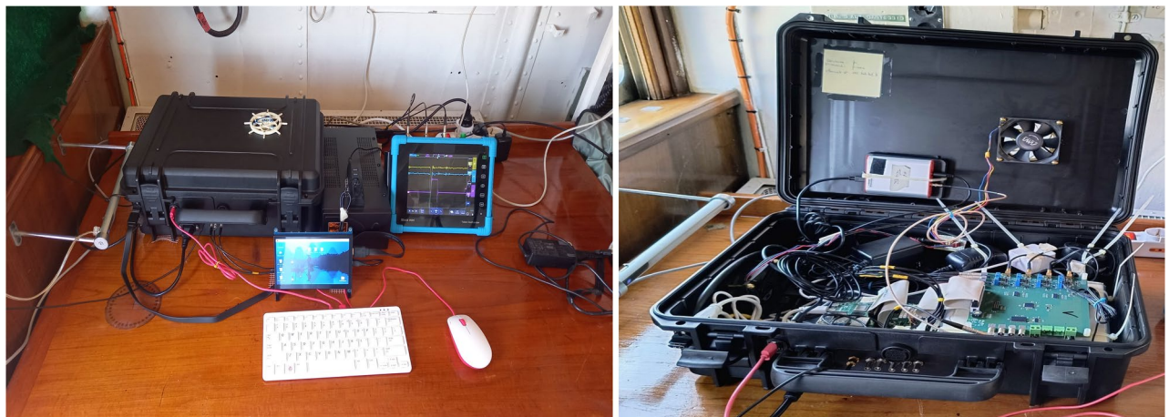
Fig. 10. Left panel: the detector box installed on a desk in the Vespucci nautical room. Right panel: detector box inside view with electronic board, the SiPM bias module and the RPi4. The scintillator tiles are below the electronic board on the right side of the detector case.
