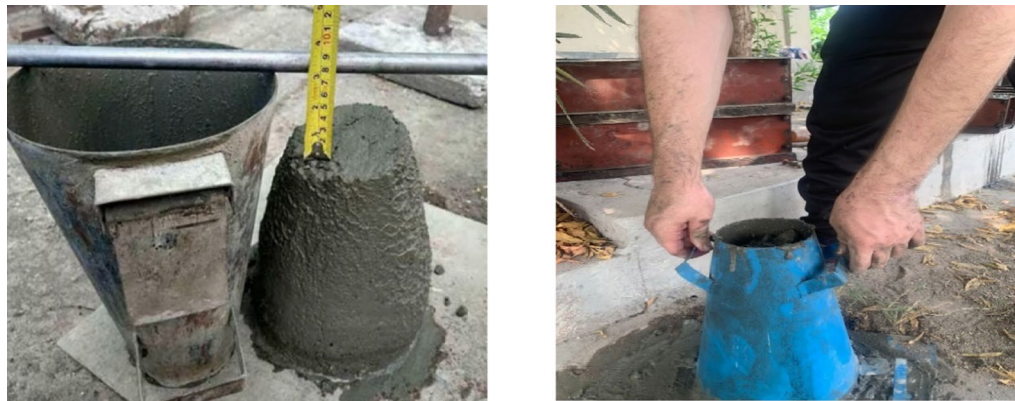
Fig. 6. Measurement of workability using the slump cone apparatus.
