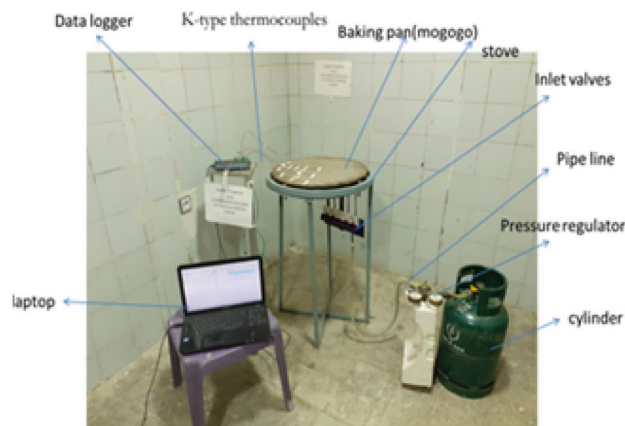
Fig. 17. Setup for temperature distribution for all material setup.
