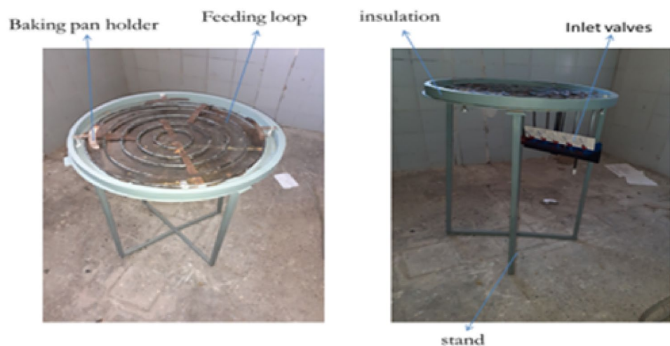
Fig. 13. Shows for improved stand stove prototype manufactured.
