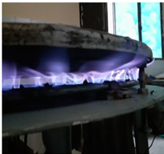
Fig. 29. Flame propagation and characteristics for flame distribution deflected by baking pan.
