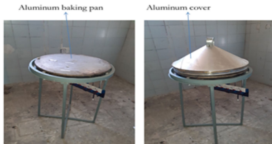
Fig. 14. Indicated for improved aluminum baking pan and cover stove prototype manufactured.
