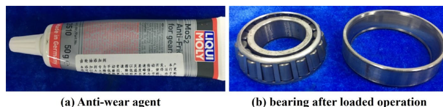
Fig. 11. Bearings operating under load after the addition of anti-wear additives.
