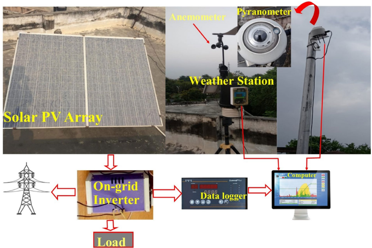
Fig. 2. Schematic diagram of the experimental setup showing the rooftop PV array and weather station connected to a data logger for real-time monitoring.
