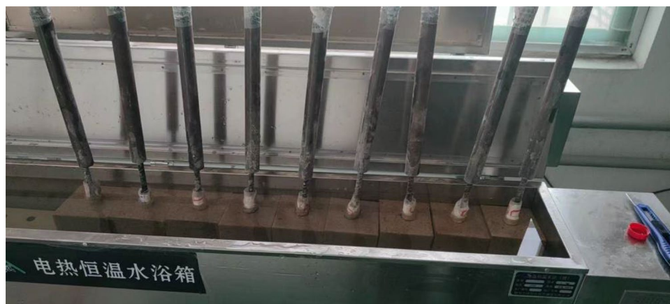
Fig. 3. Aging environment of the specimen.
