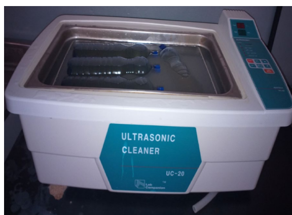
Fig. 5. Ultrasonic cleaning process.
