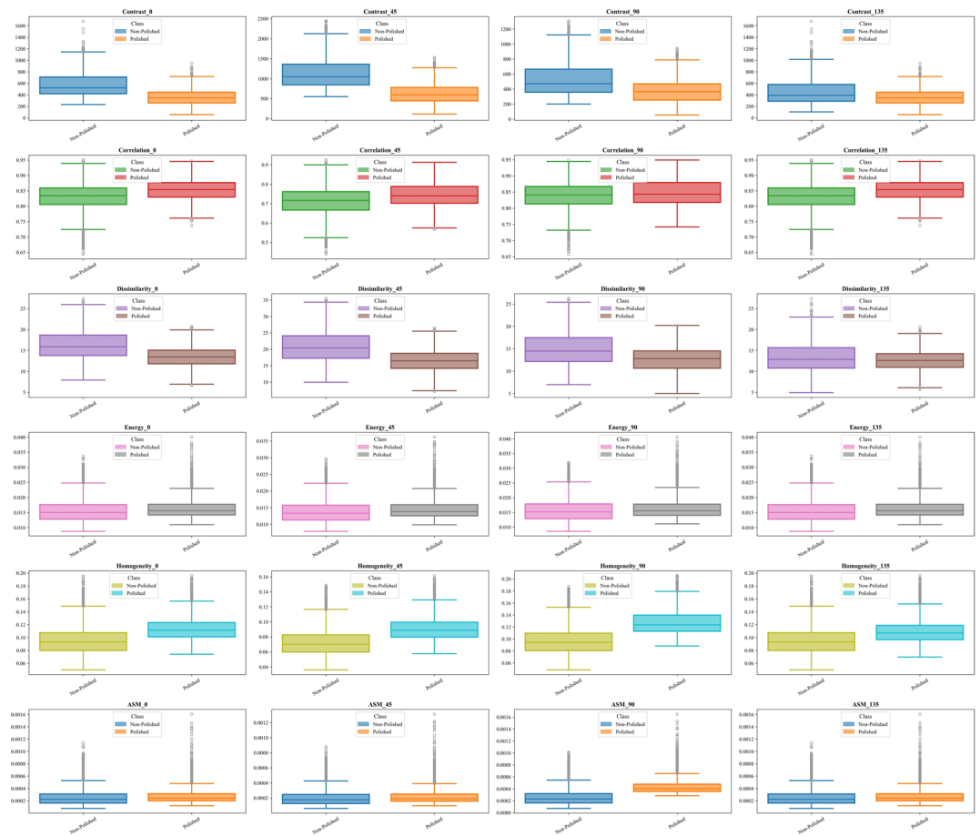
Fig. 6. Distribution of GLCM-based texture features for Non-Polished and Polished.
