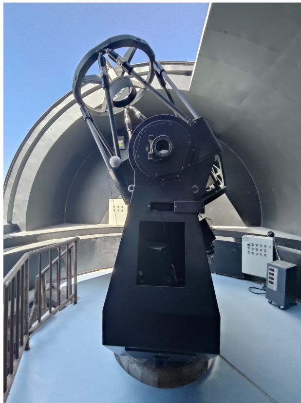
Fig. 2. MEET in its dome. This telescope has an 80 cm aperture and adopts a Ritchey-Chrétien optical structure (focal ratio f/7 ). It has one Cassegrain focus and two Nasmyth foci. A QHY600 scientific-grade back-illuminated CMOS camera is configured at one of the Nasmyth foci. It has a field of view of 22.1' \times 14.8' , and a 5-position filter wheel is installed at this focus.
