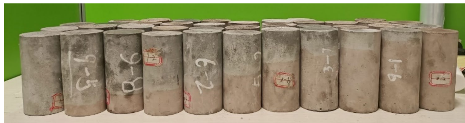
Fig. 2. Standard samples labelled and stored in an outdoor environment.
