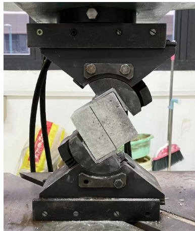
Fig. 9. Variable-angle shear test diagram.
