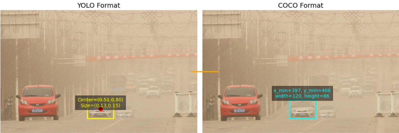
Fig. 4. Comparison of YOLO and COCO bounding box annotation formats with conversion mapping.
