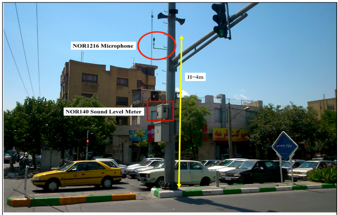
Fig. 3. Measurement and surrounding environment at fixed sound measurement stations.
