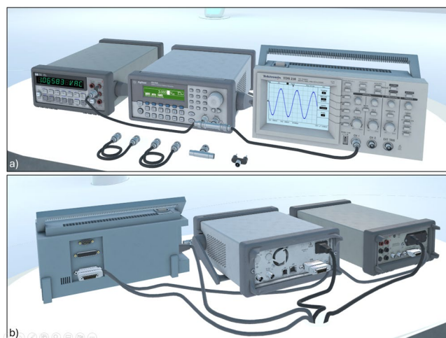
Fig. 2. The measurement setup consists of an arbitrary waveform generator, a digital multimeter and a digital storage oscilloscope, the fundamental instruments for most measurements and instrumentation courses. Instruments representation (a) Front View (b) Back View.
