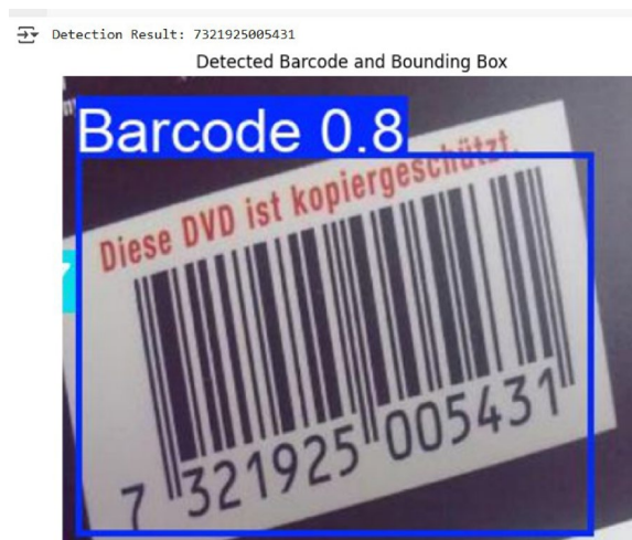
Fig. 15. Decoding the detected barcode using OpenCV.
