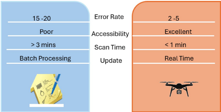
Fig. 1. Comparing traditional methods versus drone-powered inventory management.
