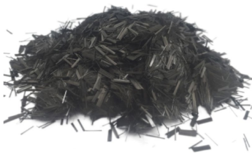
Fig. 1. 20 mm chopped carbon fiber.
