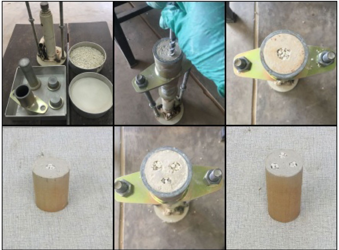
Fig. 2. Preparation and installation of polypropylene columns for both single and group columns.
