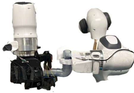
Fig. 3. Dexterous hands for pipe assembly. Image source; Informatics, Cobots and Intelligent Construction Lab, University of Florida .
