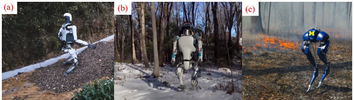
Fig. 4. Humanoid robots for operating hazardous areas: (a) DR01 walk through gravel. Image Source 9 ; used with permission; (b) Atlas HD walks through snow. Image Source 4 ; used with permission; (c) Cassie Blue walks through fire. Image Source, Michigan Robotics: Dynamic Legged Locomotion Lab 149,154 .
