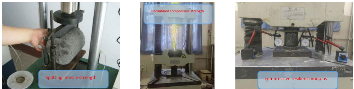
Fig. 3. WAW-300 hydraulic servo universal testing machine and control system.
