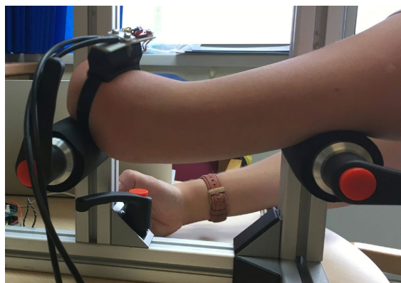
Fig. 7. The arm of the subjects was either in a relaxed hanging position besides the body or resting on a frame while the motor was placed on three different positions (the distal and proximal tendon and the muscle belly) of the biceps brachii.
