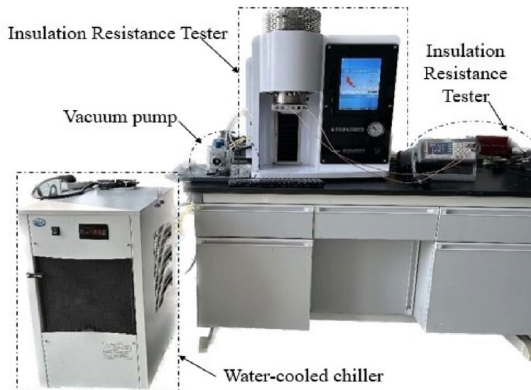
Fig. 2. Testing system of high temperature insulation resistance.
