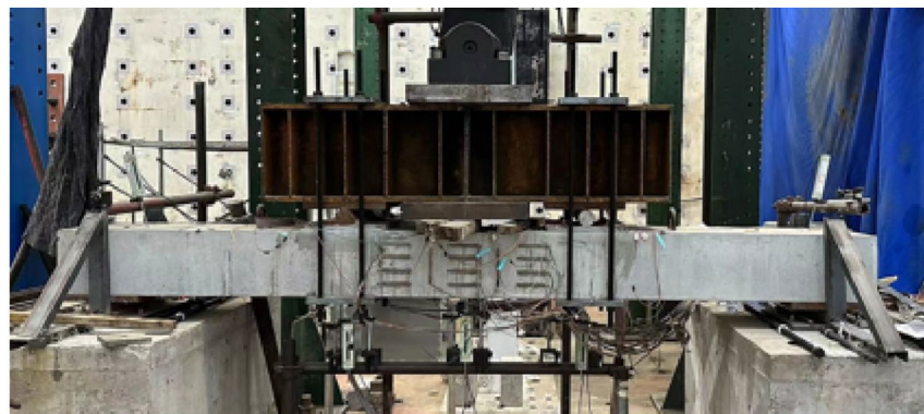
(a) Fatigue loading test of RC.
