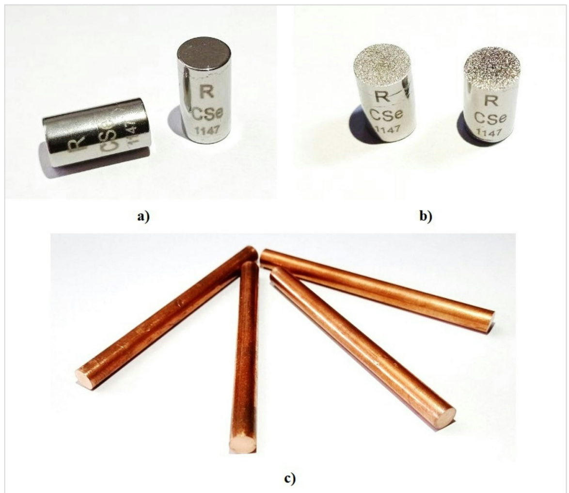
Fig. 2. (a) Workpiece before machining, (b) Workpiece after machining, (c) Copper electrodes used in experiments.
