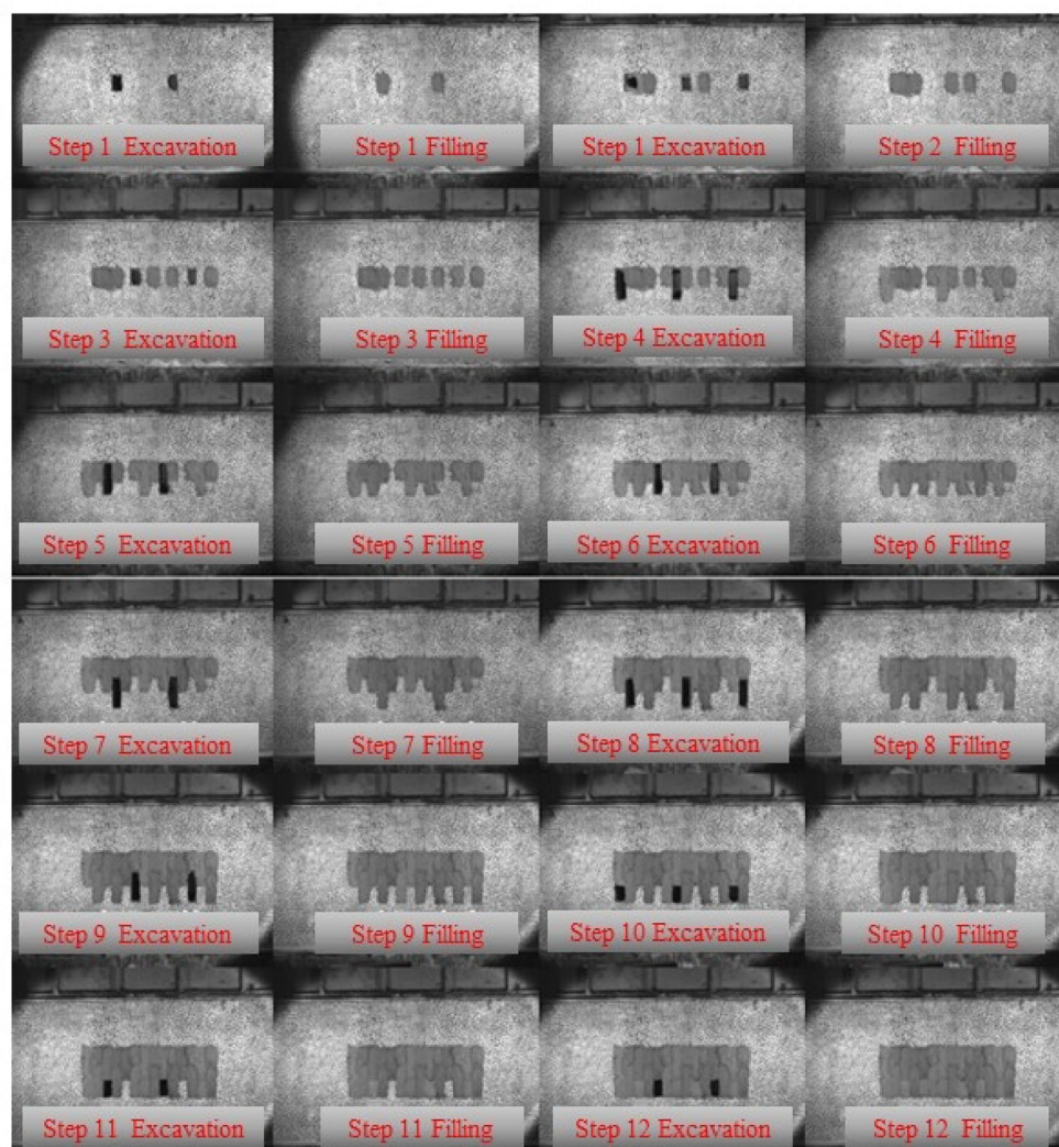
Fig. 7. Diagram of the excavation-filling sequence used in the physics model test.
