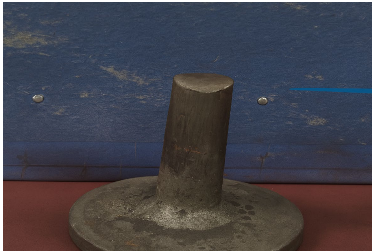
Fig. 6. Total length undersize defect.
