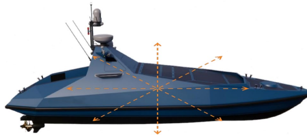
Fig. 3. Schematic illustration of the discrete action space. Arrows indicate the eight permissible motion directions in the horizontal plane, uniformly distributed at 45^\circ intervals.
