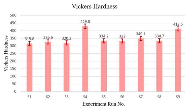
Fig. 10. Average hardness values of Fe-V 2 AlC-GO composite.
