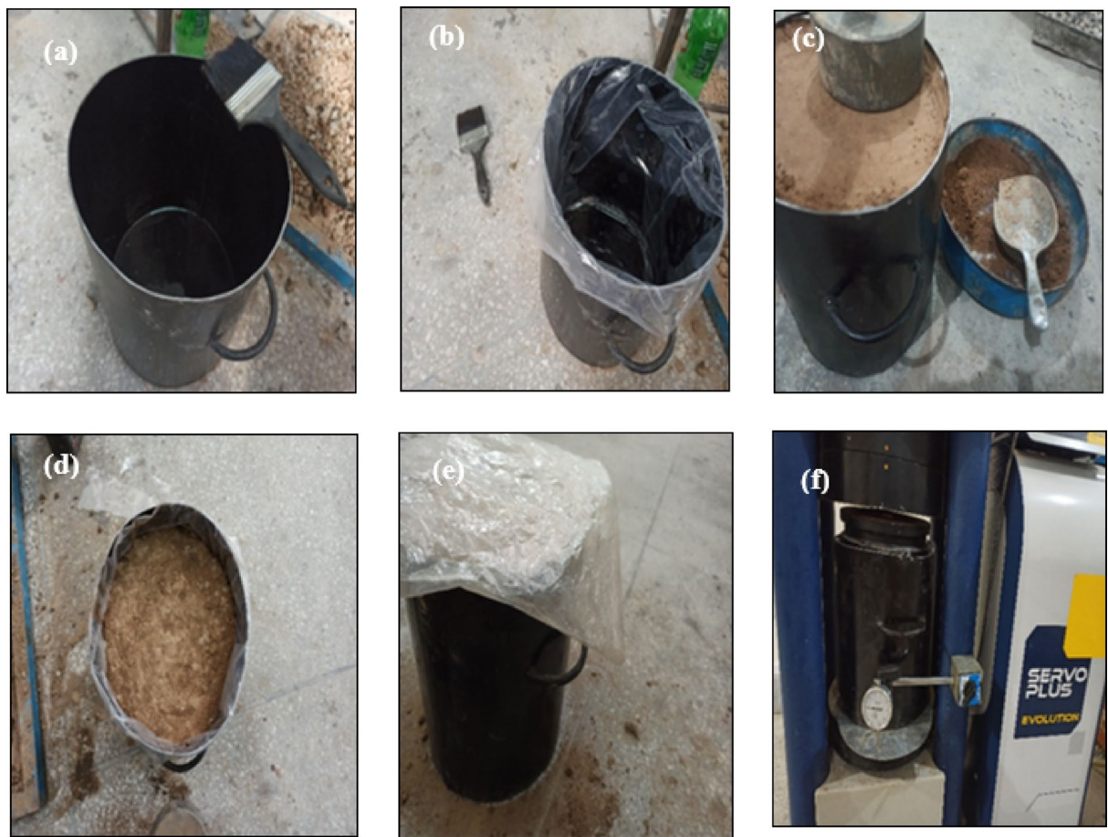
Fig. 6. Stepwise preparation of soil samples for model testing: (a) tank lubrication, (b) plastic sheet placement, (c) soil compaction, (d) prepared sample, (e) curing process, and (f) testing under hydraulic compression machine.
